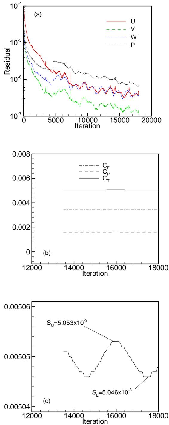
Figure 3. Iteration history for Series 60 on grid 1: (a) solution change, (b) ship forces -  $C_F$ ,  $C_P$ , and  $C_T$  and (c) magnified view of total resistance  $C_T$  over last two periods of oscillation.
